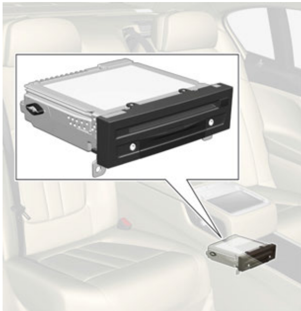
RSE control unit in combination with Lounge equipment Installation location of RSE control unit
